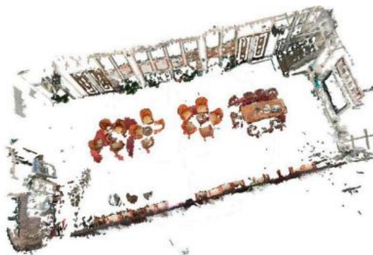
Fig 4. Reconstructed model of a meeting room using hierarchical SfM method
