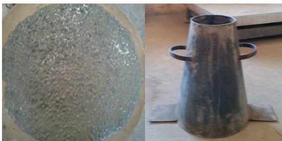
Fig. 2. Slump flow test and apparatus
