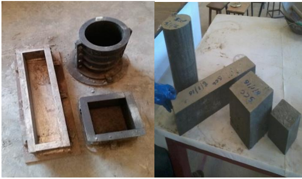
Fig. 5. Moulds and casted specimen
