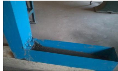
Fig 6. Concrete flows through L- box
