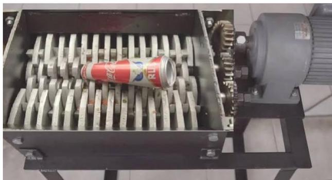
Fig 5. Plastic shredder/crusher machine
