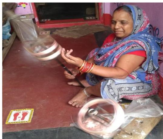
Fig. No .2 – 'Nataa' and 'Chadiki' used for divide yarn to warp and its winding
