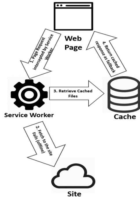
**Fig. 2. Working of Service Worker when Offline**
