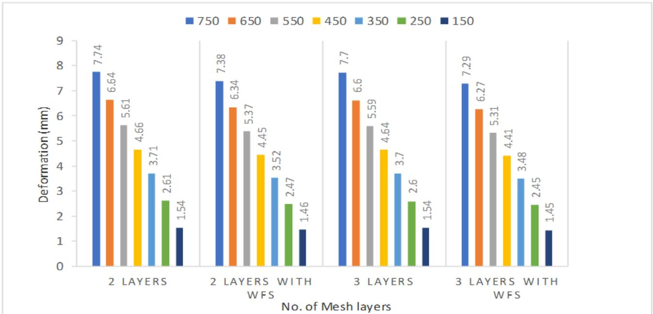
Graph 1: Deformation in (mm) For 15mm thick Ferrocement Panel.
