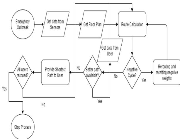
**Fig 2:Flow of control during evacuation**
