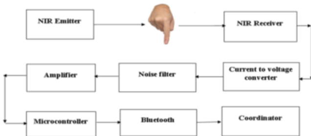
Figure 3.2: Block Diagram of Sugar level monitoring module
