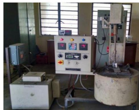
Fig. 1. Stir Casting Process Set-Up
