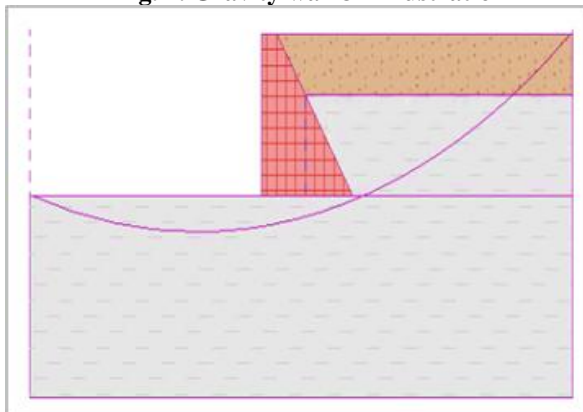
Fig. 3. Gravity wall stability analysis
