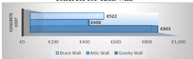
Fig. 12. Comparative cost chart of required concrete
