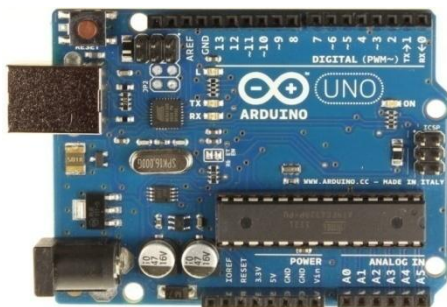
Fig. 2. Arduino Uno Microcontroller AT Mega 328P
