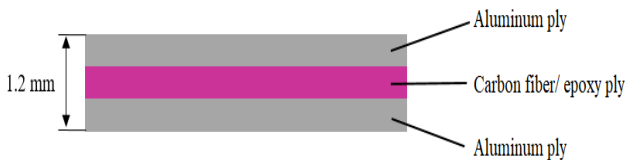
Fig. 1.Schematic diagram of 2/1 CARALL
