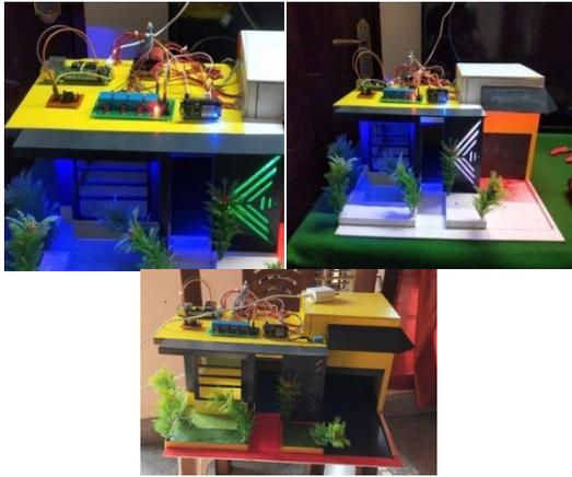
**Fig 10: Output Of Home Automation System When One Relay Is Turned On and Off**
