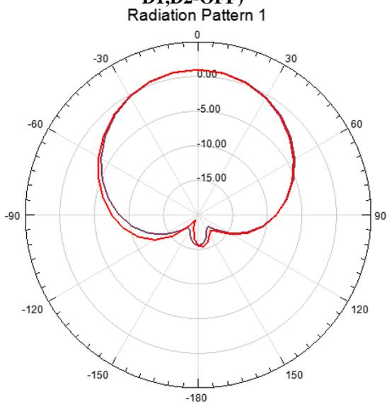
Fig.15 Proposed reconfigurable antenna Radiation pattern 2.43GHz (Two diodes D1, D2-OFF)
