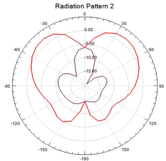
Fig.16 Proposed reconfigurable antenna Radiation pattern 5.11GHz (Two diodes D1, D2-OFF)
