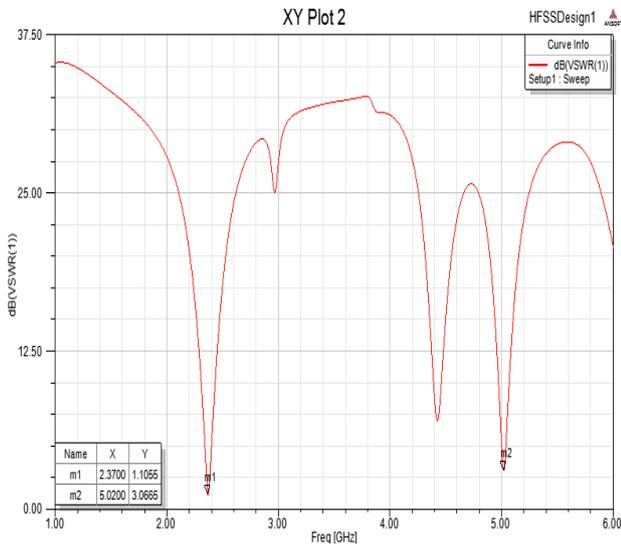
Fig.13 Proposed reconfigurable antenna VSWR 2.3 and 4.99GHz (Both the diode D1, D2 turns ON)
