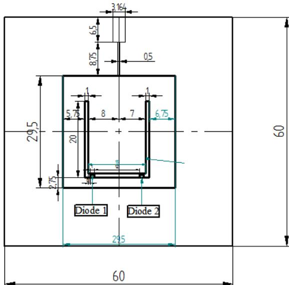
Fig. 7 Proposed Reconfigurable Antenna
