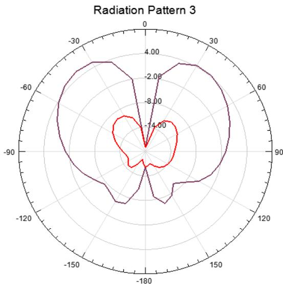
Fig.21 Proposed reconfigurable antenna Radiation pattern 4.98GHz (Diodes D1-ON and D2- OFF)
