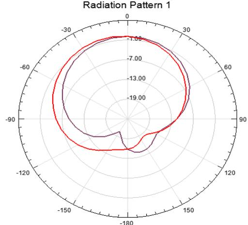
Fig.24 Proposed reconfigurable antenna Radiation pattern 2.2GHz (Diodes D1-OFF and D2- ON)
