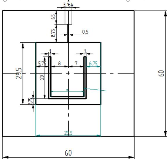
Fig.4 Modified Using U-Slot
