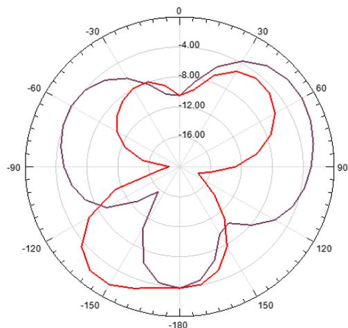
Fig.12 Proposed reconfigurable antenna Radiation pattern 4.99GHz (Both the diode D1, D2 turns ON)
