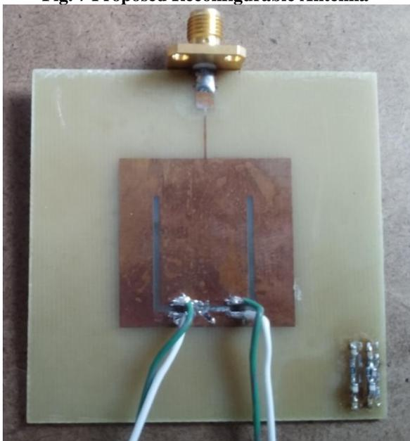
Fig.8 Experimental Measuring U-slot Antenna
