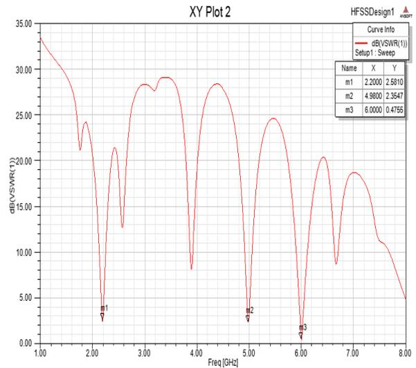
Fig.22 Proposed reconfigurable antenna VSWR 2.2, 4.98, 6GHz (D1-ON, D2- OFF)
