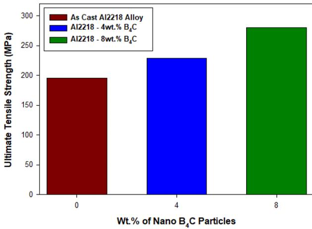
Fig. 6 Showing the ultimate tensile strength of Al2218 alloy-4 and 8 wt.% B<sub>4</sub>C nano composites
