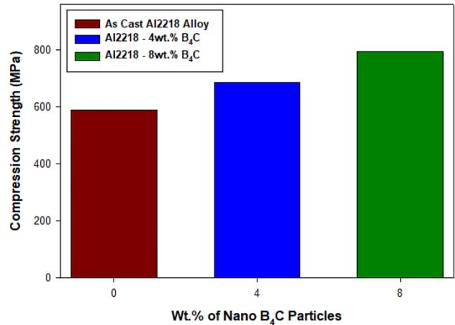
Fig. 9 Showing the compression of Al2218 alloy-4 and 8 wt.% B<sub>4</sub>C nano composites
