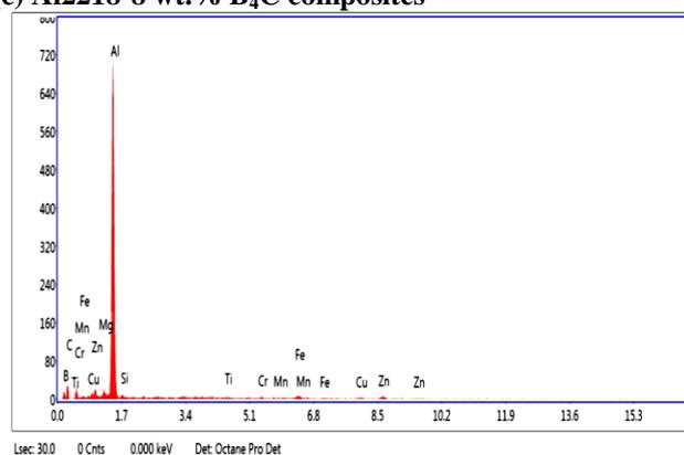
Fig. 2 Showing the EDS of Al2218-8 wt. % B<sub>4</sub>C composites
