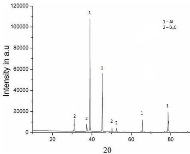
**Fig. 3 XRD pattern of Al2218- 8 wt. % of nano B<sub>4</sub>C composite**
