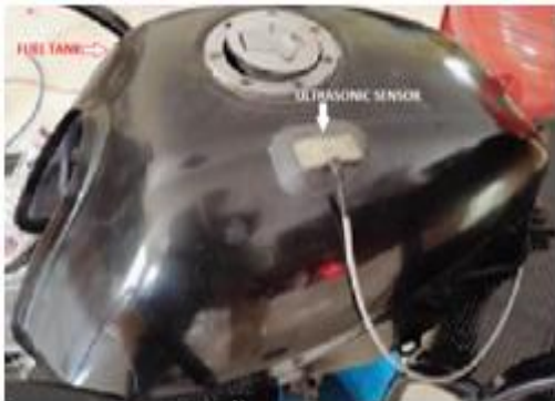
Figure 11: Developed prototype of Fuel Level Indication System
