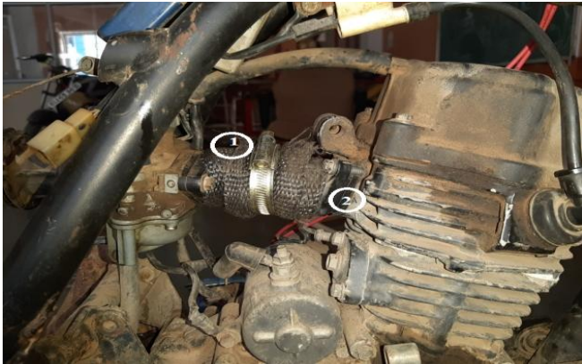
Fig 3. Insulation on the intake manifold, 1. Titanium exhaust
