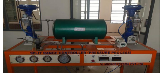
Fig.1 Pressure process station.
