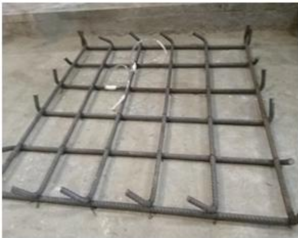
12.a) Strain Gauges of Conventional Deformed Steel Bars Reinforcement
