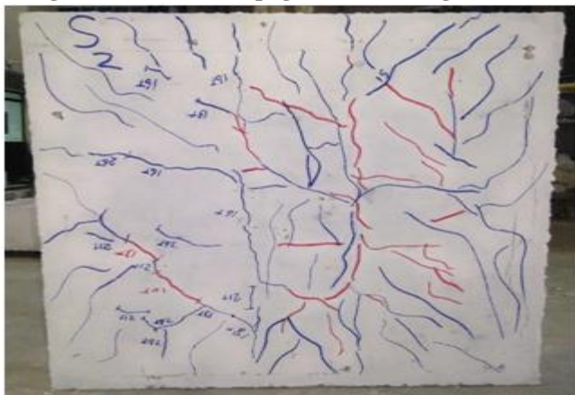
Figure 14: Cracks Propagation of Testing Slab (S2)
