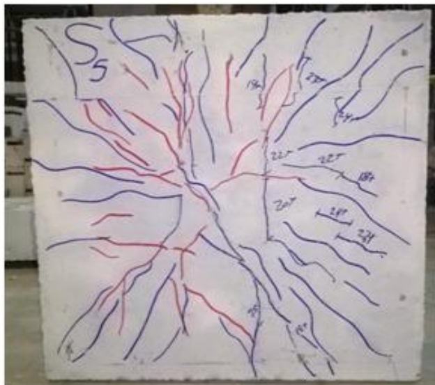
Figure 17: Cracks Propagation of Testing Slab (S5)
