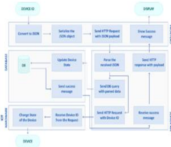
Fig. 3: Functional Architecture: Device Control
