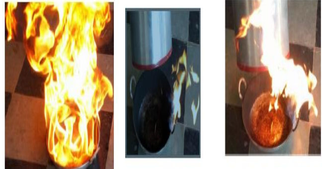
Figure 1.9: Testing of Sound Wave Fire Extinguisher Testing of the Portable Sound Wave Fire Extinguisher on Liquid Fire.
