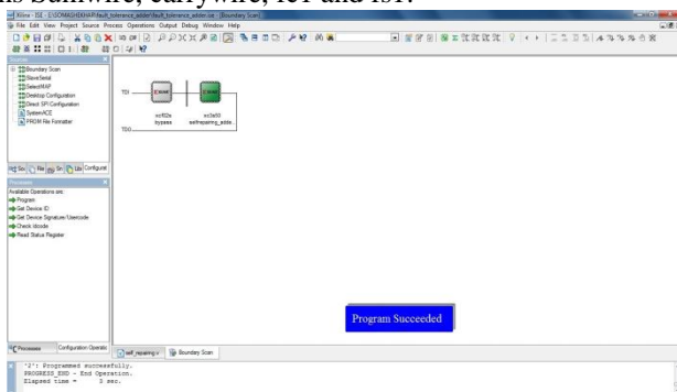
Fig 10. Boundary Scan checking
