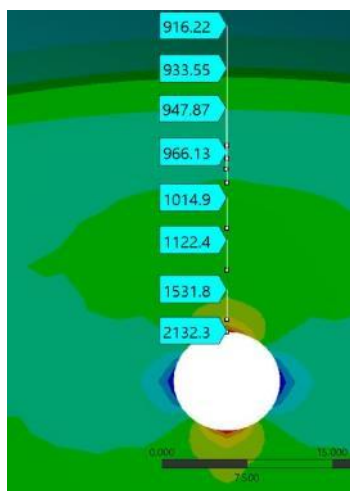
Fig. 32. Hoop stress variation along surface at 45000 RPM
