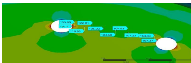
Fig. 16. Radial stress variation along the corner at 15000 RPM
