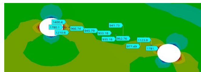
Fig. 28. Radial stress variation along the corner at 45000 RPM
