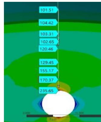
Fig. 19. Hoop stress variation along surface at 15000 RPM
