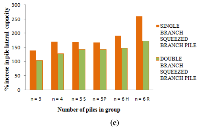
Figure 8: Percentage Increment in (a) Ultimate load capacities of squeezed branch pile group with number of piles in the group, (b) Ultimate uplift load capacities of squeezed branch pile group with number of piles in the group, and (c) Ultimate lateral load capacities of squeezed branch pile group with number of piles in the group
