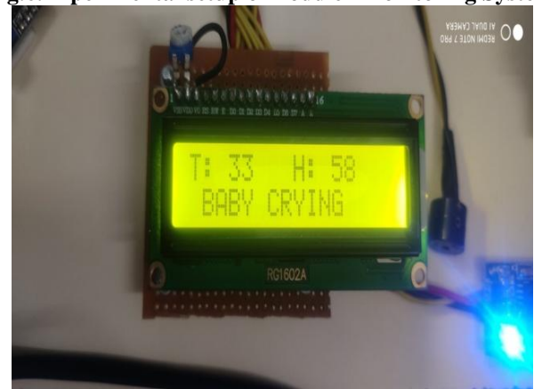
Fig.7.Measuring of temperature and humidity along with displaying whether baby crying or not
