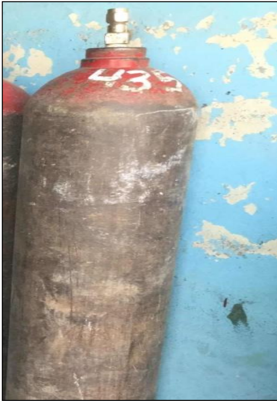
Fig 3. Nitrogen gas cylinder (140 psi pressure)
