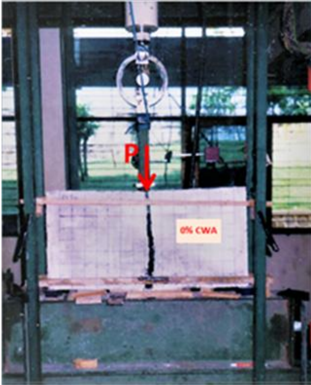
Fig. 7. The crack pattern of normal concrete panels (0% CWA)
