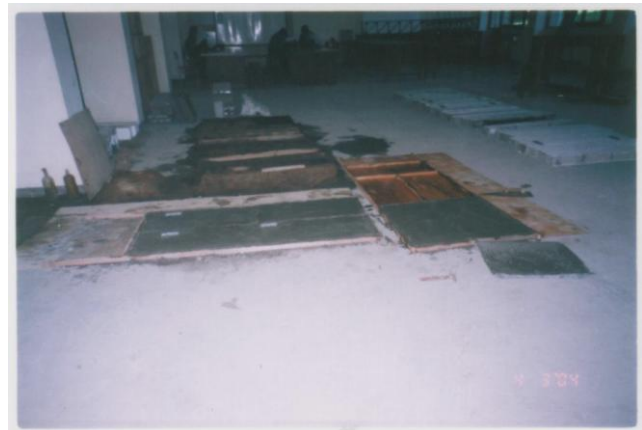
Fig. 4. Manufacture of panel test specimens
