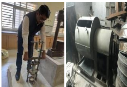
Fig. 3: Laboratory setup and Equipments for AIV and LAAV tests (IS: 2386-Part 4)
