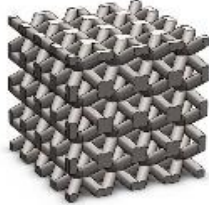
Fig. 1. Schematic of lattice structure cube specimen.
