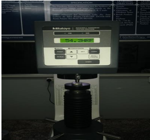
Fig. 4. Hardness test on Rockwell hardness testing machine
