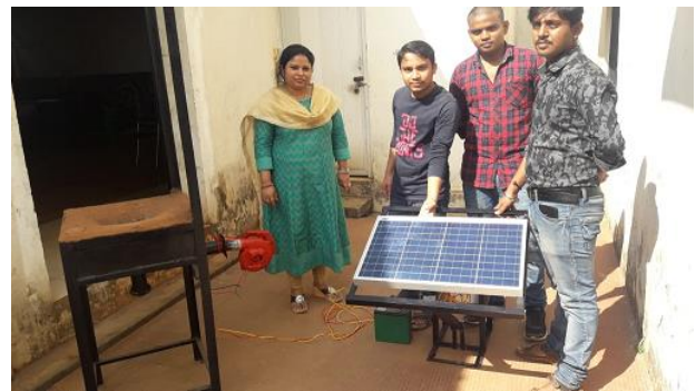
Figure 6. Full assembly of solar operated blower for forging operation
