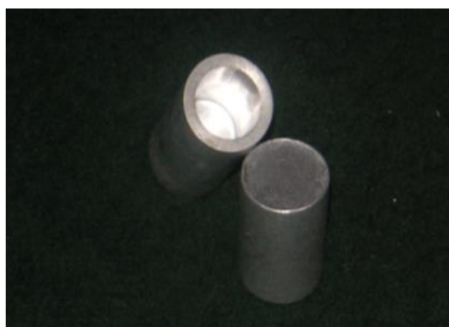
Fig.3 Photograph of Slug and extruded tube
