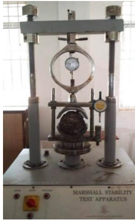
Figure 5, Marshall Stability test on samples
