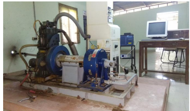
Fig.-I: Computerized VCR Engine Setup with Smoke meter and Gas analyzer.
