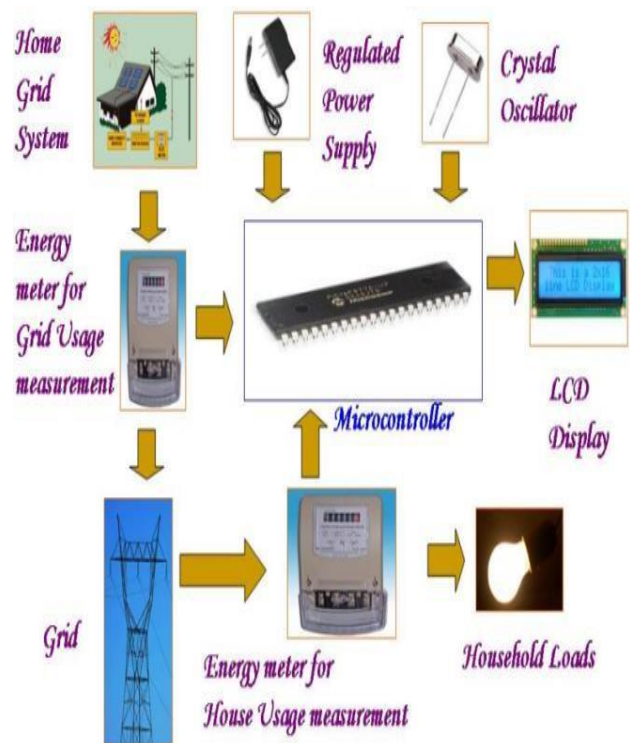
Fig. 1. Block diagram of net energy metering system with hybrid energy storage system
