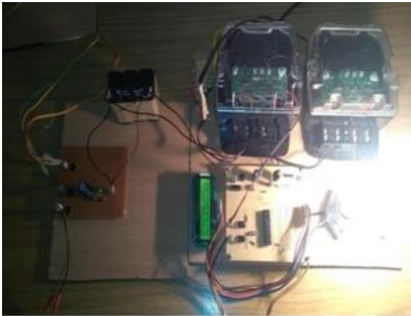
Fig. 7.LCD displaying the net energy
