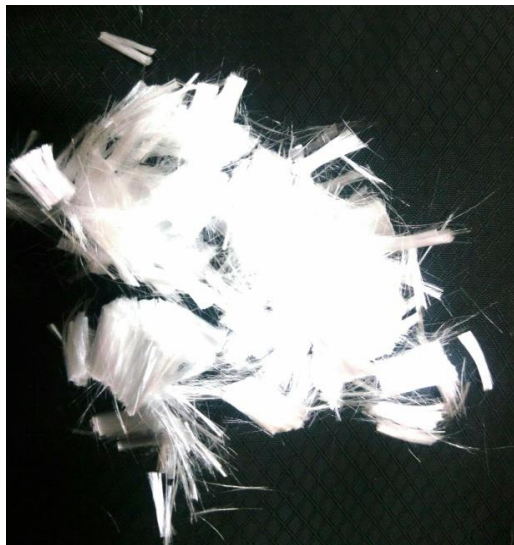
Fig.1. Polypropylene fiber (monofilament form)
