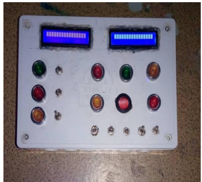
Figure 4: The Implemented hardware human machine interface Model for the Smart Microgrid Power Pool System
