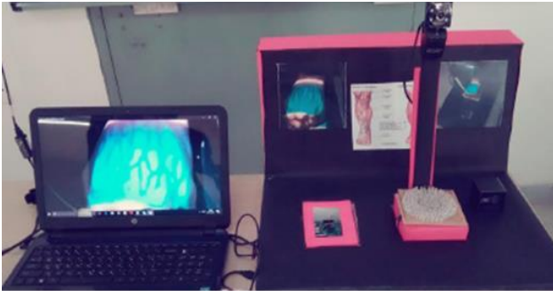
Fig 8: Working model of NIR Based Accuvein
