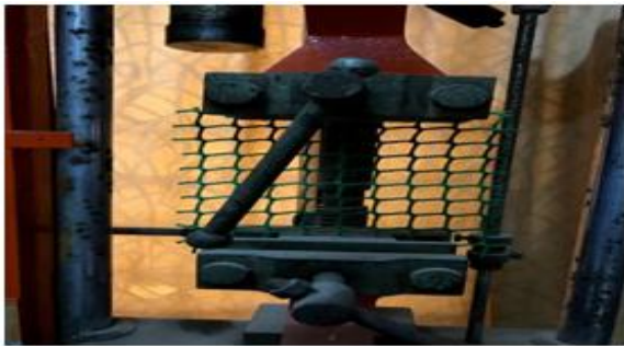
Fig. 3 Geogrid - Before Load Application
