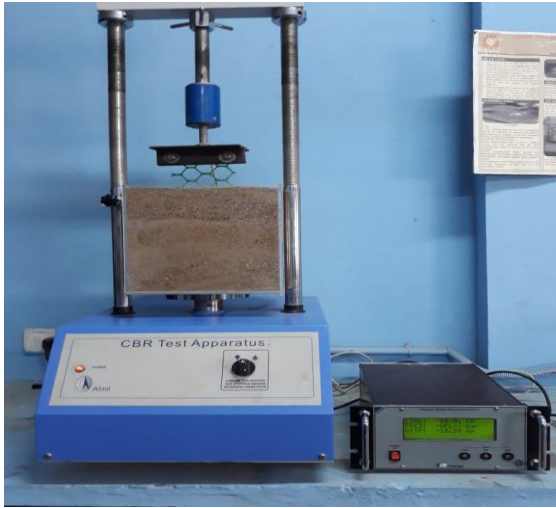
Fig. 5 Experimental setup for pullout test
