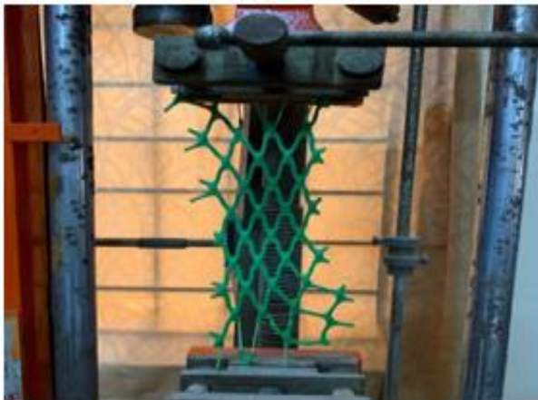
Fig. 4 Geogrid at failure
