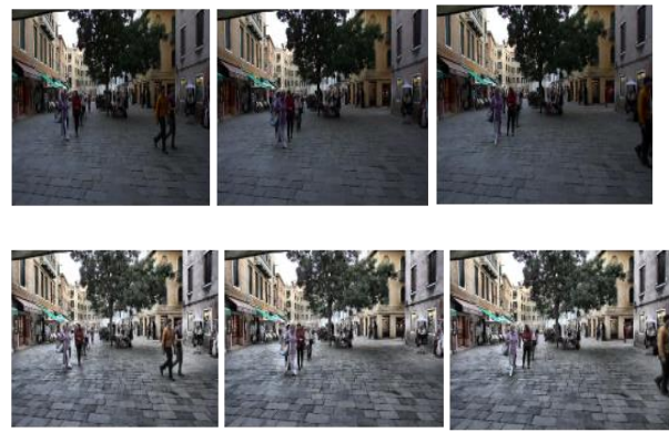
Fig.4. Selective Frames 1,2,3 Input and Enhanced Output Frames with CLAHE_LUV color space. The performance metric used to measure the quality enhancement here is the average entropy [27]-[30] value for the sample frames. Entropy measure is the No reference Image Quality assessment metric and higher the value, the richness of details is much more. Here Fig.5 illustrates the visual representation of performance metric, entropy measure for selected frames and the entropy value for selected frames with CLAHE_LUV has shown better improvement.
