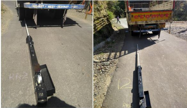
Fig. 3. Benkelman Beam Deflection study on selected stretches
