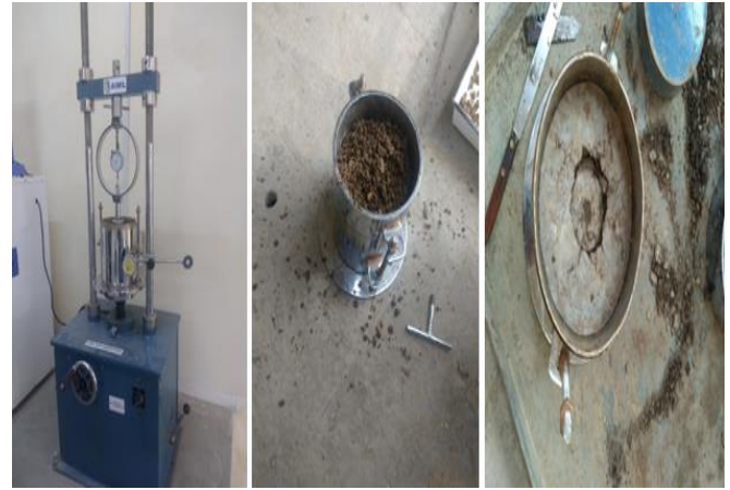
Fig. 5. California Bearing Ratio Test in Laboratory
