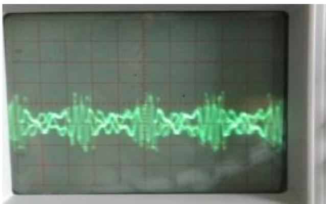
Figure 16. IIR filter output for input signal frequency= 4KHz
