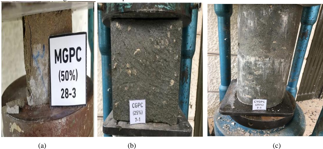
Figure.2: Resistance strength experiments for (A) Masonry cubes with 50% Phosphorite wastes and 50% Gypsum, (B) Phosphorite wastes fine and Gypsum concrete cubes, (C) Phosphorite wastes fine Gypsum concrete cylinders.
