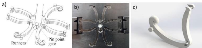
Fig. 1. (a) Design of Cavities for Microinjection Molding (b) Cavities and Sliders, and (c) Polymer Ligation System
