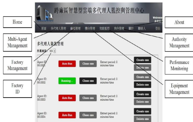
Fig. 9. Injection molding machine manufacturing monitoring system interface.
