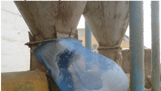
Figure 1. Deterrence of fiber waste from VZP-type dust collector at the Metan Cotton Ginning Plant in Samarkand Region
