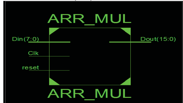
Fig 4: Array Multiplier RTL Schematic Report
