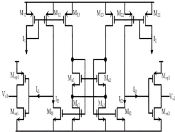
**Fig. 7. CMOS circuit design of WTA Network**
