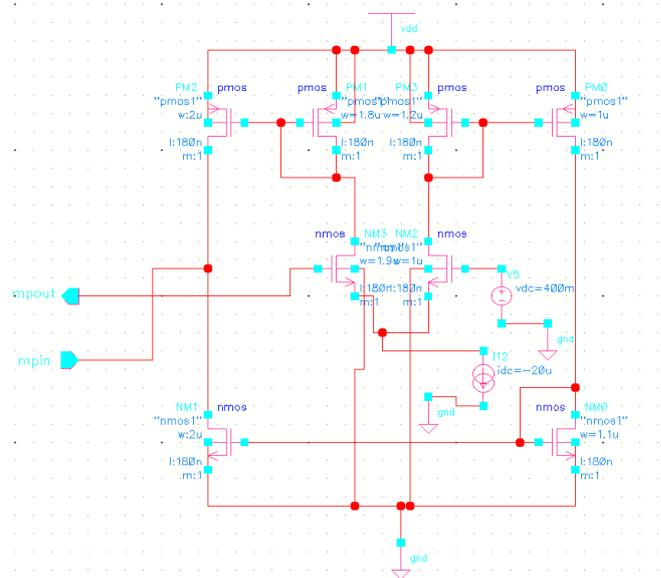
**Fig 10: The schematic circuit of mapping circuit in cadence**
