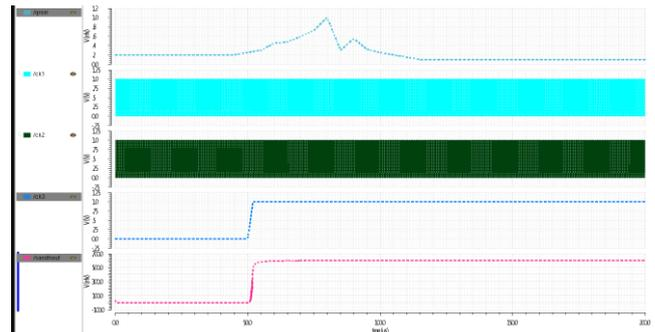
**Fig 9: Transient response of Sample and Hold circuit**
