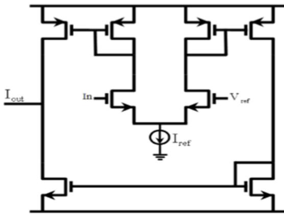
Fig. 3. CMOS circuit design of Mapping circuit
