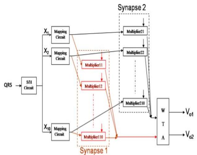
Fig. 1. Block diagram of arrhythmia classifier
