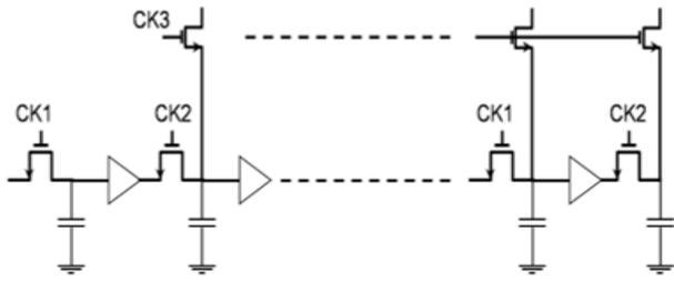
Fig. 2. CMOS circuit design of sample and hold circuit
