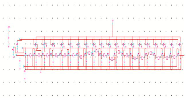
**Fig 8: Schematic diagram of Sample and Hold circuit in Cadence**
