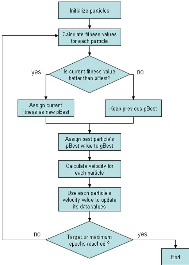
Figure 7.1 Flow diagram illustrating the particle swarm optimization algorithm.
