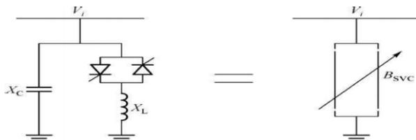
Fig 2.1 SVC Structure and variable shunt susceptance.
