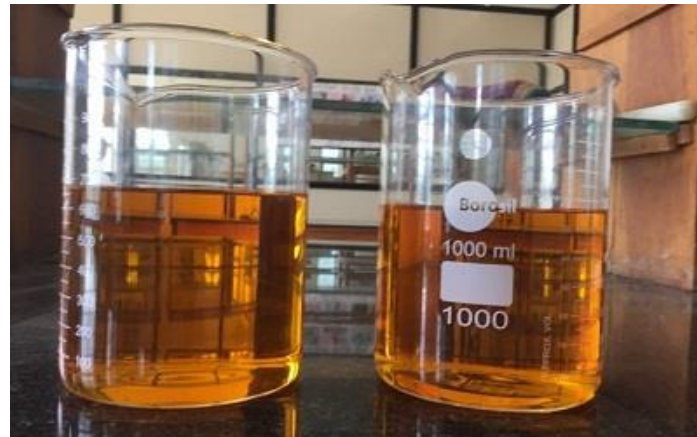
Fig. 4. Biodiesel after drying
