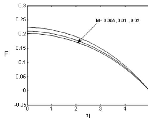
Figure 2. Effect of  $M$  on velocity profiles of particle phase for  $\varepsilon = 5.0, \beta = 0.03, \phi = 0.01, \gamma = 1200,$
