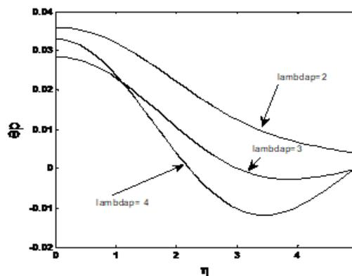
Figure 3. Effect of  $\lambda_p$  (loading ratio) on velocity profiles of particle phase for  $\varepsilon = 5.0, \beta = 0.03, \phi = 0.01, \gamma = 1200,$
