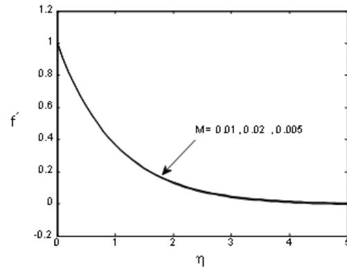
Figure 1. Effect of  $M$  on velocity profiles of carrier fluid phase for  $\varepsilon = 5.0, \beta = 0.03, \phi = 0.01, \gamma = 1200,$
